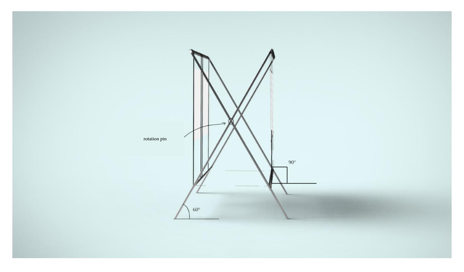
The structure is 60-degree tilt in relation to the floor, that allows the observer to have a better vision of the paper above.
